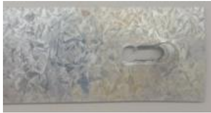
Fig. 12. Effects of T on failure modes of specimen Series 190-D-5d (a) 300 °C
