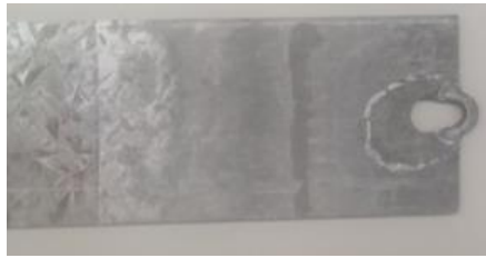
Fig. 11. Effects of T on failure modes of specimen Series 190-D-d (c) 600 °C
