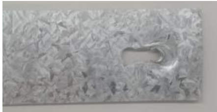
Fig. 8. Effects of e_1 on failure modes of specimen Series 190-D at ambient temperature (c) 190-D-5d
