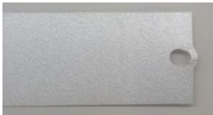
Fig. 7. Effects of e_1 on failure modes of specimen Series 042-D at ambient temperature (a) 042-D-d
