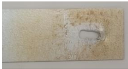
Fig. 10. Effects of T on failure modes of specimen Series 042-D-5d (a) 300 °C
