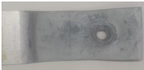
Fig. 10. Effects of T on failure modes of specimen Series 042-D-5d (c) 600 °C
