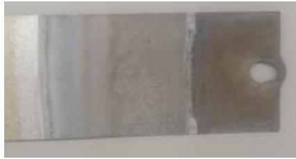
Fig. 9. Effects of T on failure modes of specimen Series 042-D-d (d) 900 °C
