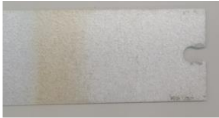
Fig. 9. Effects of T on failure modes of specimen Series 042-D-d (b) 450 °C
