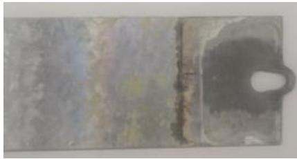
Fig. 11. Effects of T on failure modes of specimen Series 190-D-d (d) 900 °C
