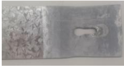
Fig. 12. Effects of T on failure modes of specimen Series 190-D-5d (b) 450 °C
