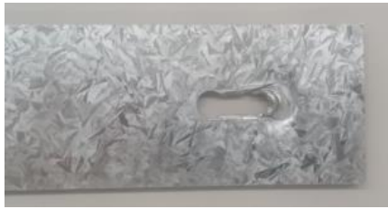
Fig. 8. Effects of e_l on failure modes of specimen Series 190-D at ambient temperature (d) 190-D-6d
