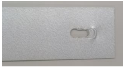
Fig. 7. Effects of e_1 on failure modes of specimen Series 042-D at ambient temperature (c) 042-D-5d
