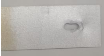
Fig. 10. Effects of T on failure modes of specimen Series 042-D-5d (b) 450 °C
