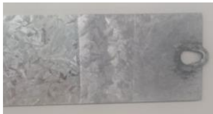
Fig. 11. Effects of T on failure modes of specimen Series 190-D-d (b) 450 °C
