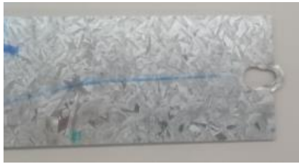
Fig. 8. Effects of e_1 on failure modes of specimen Series 190-D at ambient temperature (a) 190-D-d
