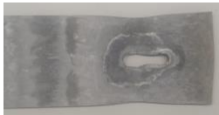
Fig. 12. Effects of T on failure modes of specimen Series 190-D-5d (c) 600 °C
