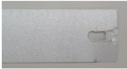
Fig. 7. Effects of e_1 on failure modes of specimen Series 042-D at ambient temperature (b) 042-D-3d
