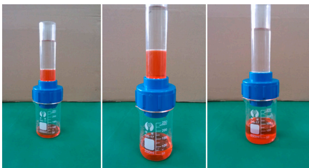
Figure 9. Oil–water separation experiment performed using the hybrid-coated mesh.
