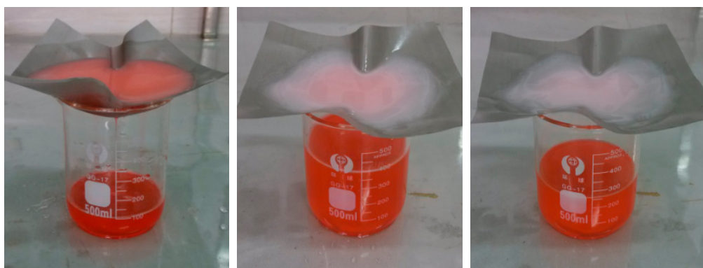
Figure 10. Renderings of membrane separation of oil and water emulsion.
