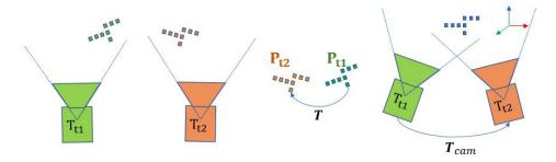
**Figure 3.** The camera pose in the world frame and the point cloud alignment procedure in the camera frame.
