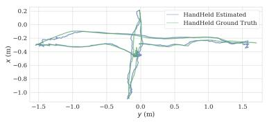
**Figure 9.** Estimate trajectory and ground truth from *x*–*y* plane of hand held test.
