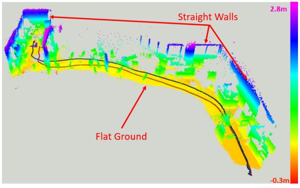
**Figure 18.** Exploration and restruction of the indoor environment using ToF–VIO, blue path (ToF–VIO), red path (T265).
