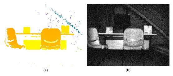
**Figure 1.** PMD Flexx ToF camera output (224 x 171 pixels). (**a**) Depth image, white color mean depth information is not available. (**b**) NIR intensity image.
