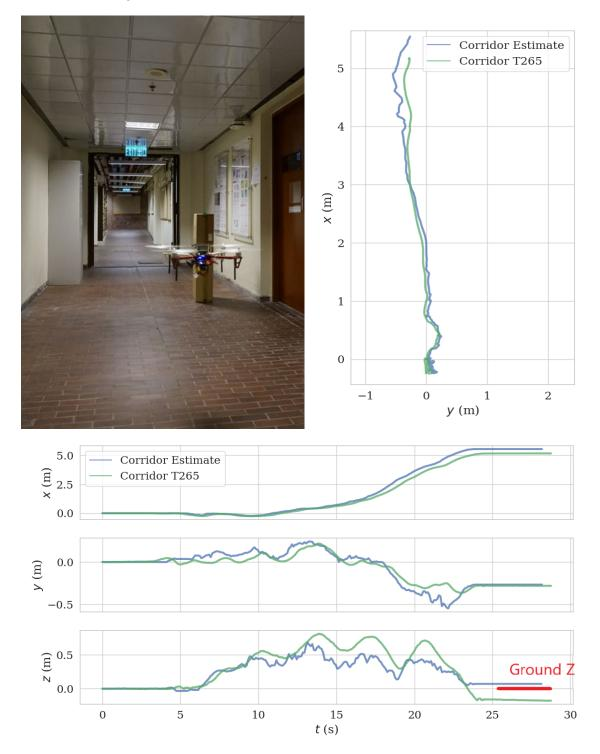
**Figure 17.** Comparison of the estimated trajectory by the current ToF–VIO sensor with that by the Realsense T265 sensor in the corridor environment.
