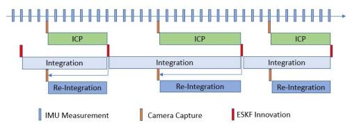
Figure 8. Time synchronization of IMU and ICP.
