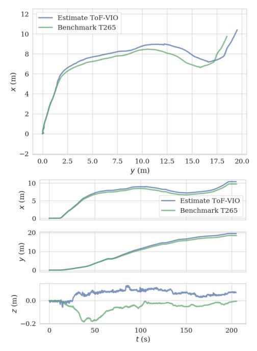
**Figure 19.** Comparison of the estimated trajectory by the current ToF–VIO sensor with that by the Realsense T265 sensor in the exploration test.
