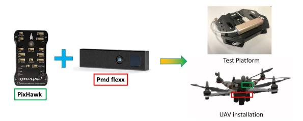
Figure 2. ToF–VIO testing platform and its implementation on a UAV.
