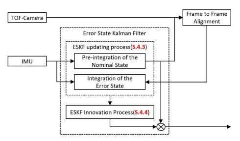
**Figure 7.** Workflow of the Error State Kalman Filter estimator by using the ToF camera alignment results and the IMU data.
