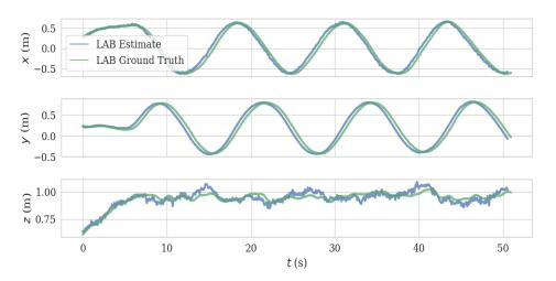
Figure 15. Comparison of estimated trajectory and ground truth of in lab environment test.
