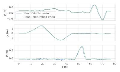
Figure 10. Comparison of estimated trajectory and ground truth of hand held test.
