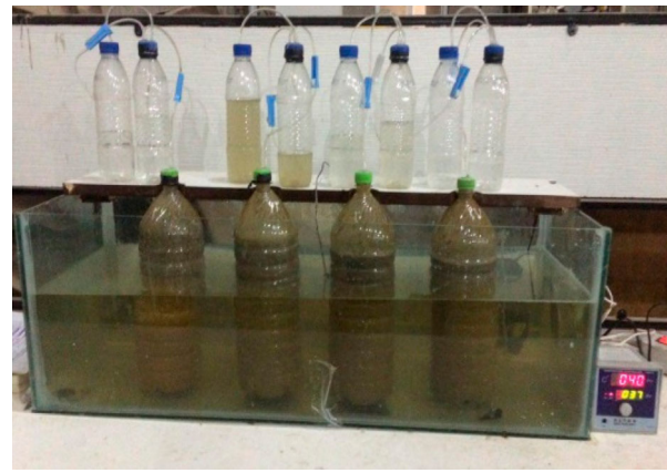
Figure 2. Biogas production and measuring setup.
