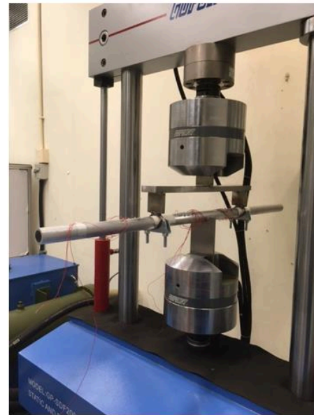
Figure 3 Steel frame combined with fatigue machine for three-point bending fatigue test
