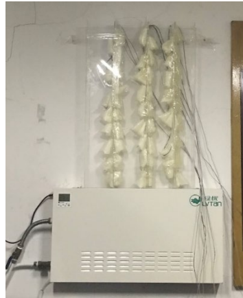
Figure 3(b). Experimental fan coil unit with the PCM duct at the outlet
