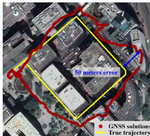
Fig. 1. Experimental UAV localization error in urban area, blue line as the true trajectory.
