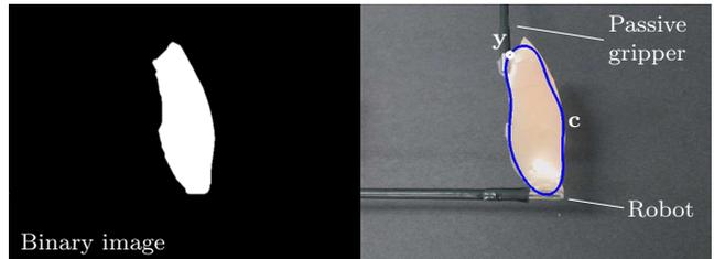
Fig. 10. The feedback contour  $c(\rho)$  computed with the captured image.
