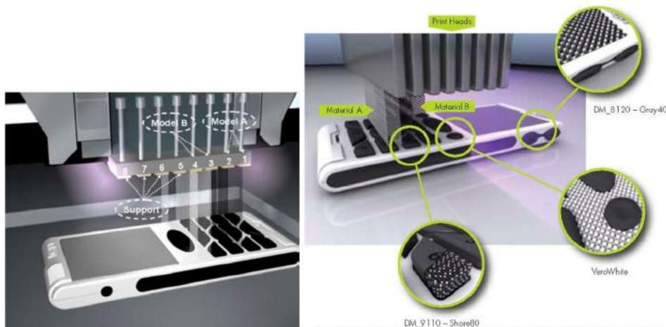
**Figure 1.** The PolyJet Matrix printing block and its working principle [10].
