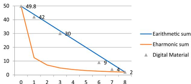
**Figure 6.** The tensile strength relationship between the digital material and the proposed material limits.
