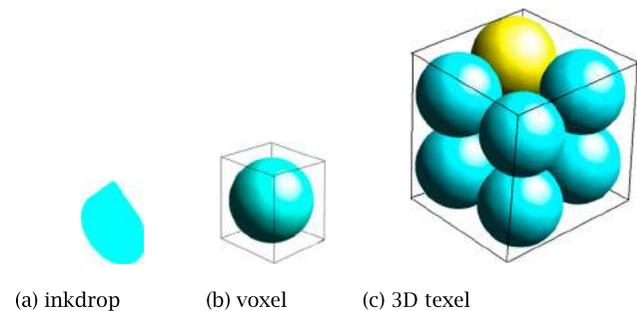
**Figure 2.** Inkdrop approximation for the formation of a composite material.
