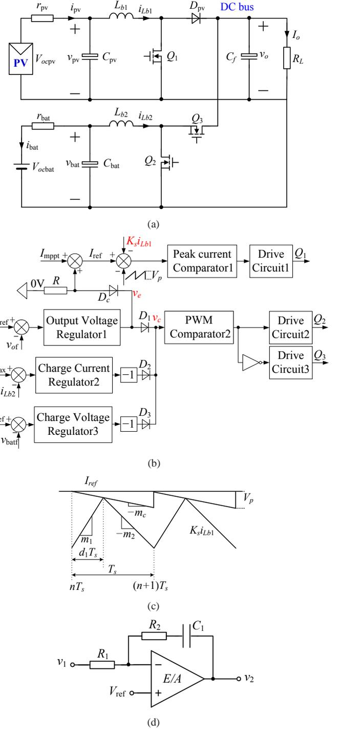
Fig. 1. Photovoltaic-battery hybrid power system. (a) Main topology; (b) control system; (c) typical waveforms for peak current control loop; (d) PI compensator.
