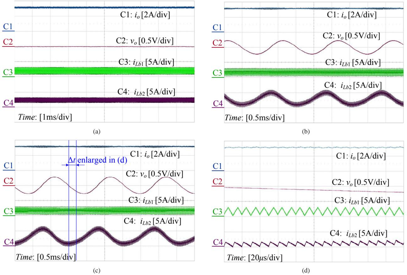
Fig. 8. Typical experimental waveforms in operating mode  $M_1$  for different values of  $V_{ocpv}$ , with  $V_{ocbat} = 38$  V,  $I_{mppt} = 0.3$  A and  $I_o = 3.3$  A kept constant. Alternating component of output voltage  $v_o$  is shown. (a) Stable period-1 operation with  $V_{ocpv} = 32$  V; (b) Neimark-Sacker bifurcation with slow-scale oscillation with  $V_{ocpv} = 26$  V; (c) coexisting fast-scale and slow-scale bifurcation with  $V_{ocpv} = 24.3$  V; (d) enlarged view of (c).
