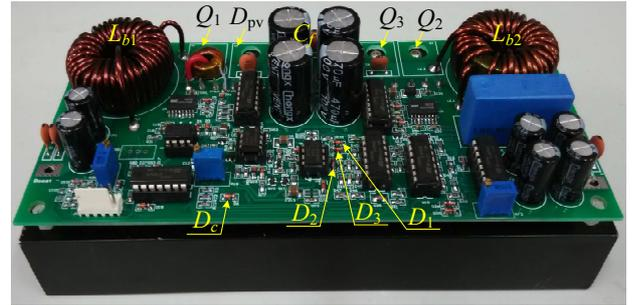
Fig. 7. Experimental prototype of multi-operating-mode PBHPS.
