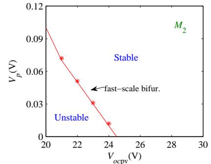
Fig. 6. Stability boundary with  $V_{ocpv}$  and  $V_p$  serving as bifurcation parameters. Points are stability boundaries obtained from circuit simulations.
