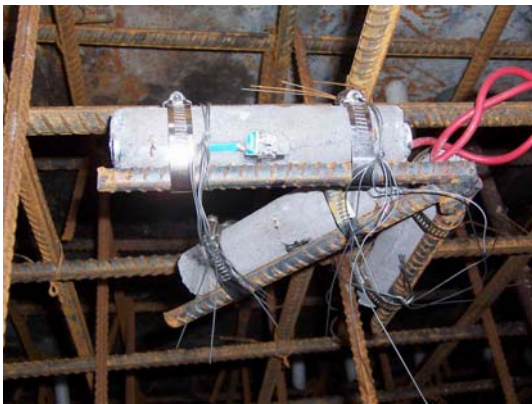
(c) A strain rosette in the inner tube
