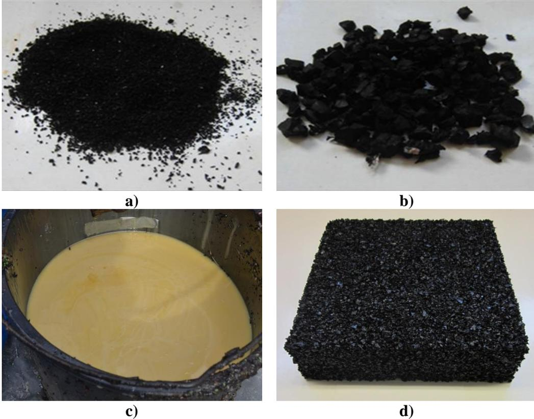
95 **FIGURE 2 Components and Test Sample of PERS: (a) Fine rubber granules; (b)**
