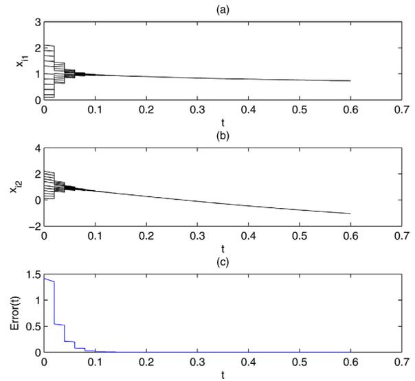
FIG. 4. (Color online) Evolution of (a) the states  $x_{i1}$ , (b) the states  $x_{i2}$  and (c) the total Error(t) of impulsively coupled systems (9) with  $\Delta = 0.02$ ,  $t_0 = 0$  and  $\theta_1 = \theta_2 = \theta_3 = 1/3, \theta_i = 0, i = 4, 5, \dots, 11$ .
