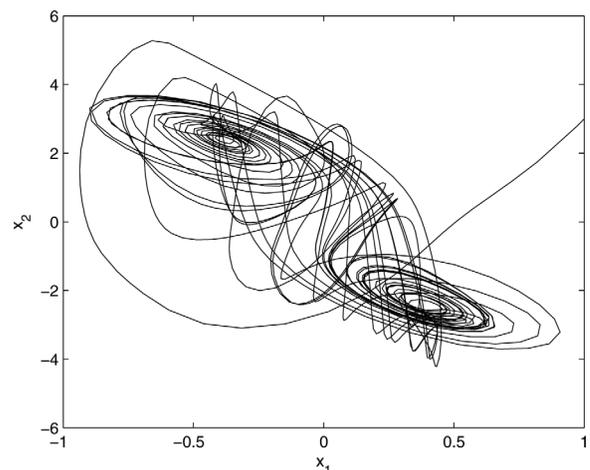
FIG. 1. A fully developed double-scroll-like chaotic attractor of delayed Hopfield neural network.
