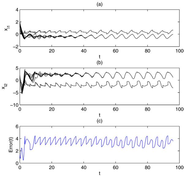
FIG. 6. (Color online) Evolution of (a) the states  $x_{i1}$ , (b) the states  $x_{i2}$  and (c) the total Error(t) of impulsively coupled systems (9) with  $\Delta = 2.2$ ,  $t_0 = 0$  and  $\theta_i = 1/11, i = 1, 2, \dots, 11$ .
