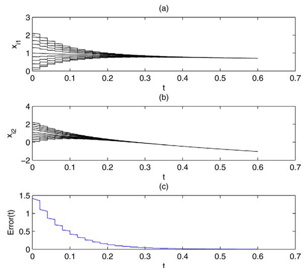
FIG. 5. (Color online) Evolution of (a) the states  $x_{i1}$ , (b) the states  $x_{i2}$ , and (c) the total Error(t) of impulsively coupled systems (9) with  $\Delta = 0.02$ ,  $t_0 = 0$  and  $\theta_1 = 1, \theta_i = 0, i = 2, 3, \dots, 11$ .
