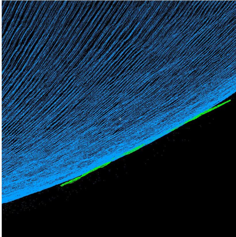
**Figure 13. Profile view of the DEM from the Backward – Nadir pair (green) overlaid on the LA data (blue).**
