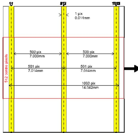
Figure 11. Chang'E1 CCD sensor geometry.
