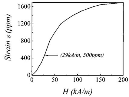
FIG. 3. Measured dependence of the effective magnetostrictive strain on the magnetic bias.
