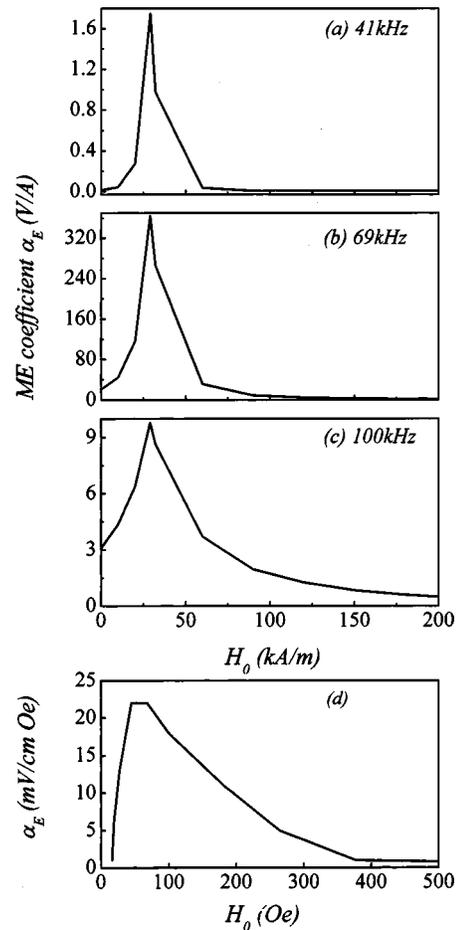
FIG. 7. Numerically calculated magnetoelastic coupling coefficient as a function of the magnetic bias field  $H_0$  at different frequencies of the ac magnetic signal: (a) 41, (b) 69, and (c) 100 kHz, respectively; (d) the experimentally measured coupling coefficient  $d$  as a function of  $H_0$  (see Ref. 7).
