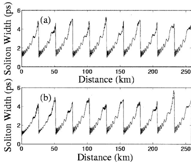
Fig. 11. Pulse width evolution under conditions identical to those of Fig. 9(b) except that the input pulse width to the first NALM is varied for (a) 4.71 ps and (b) 5.35 ps.
