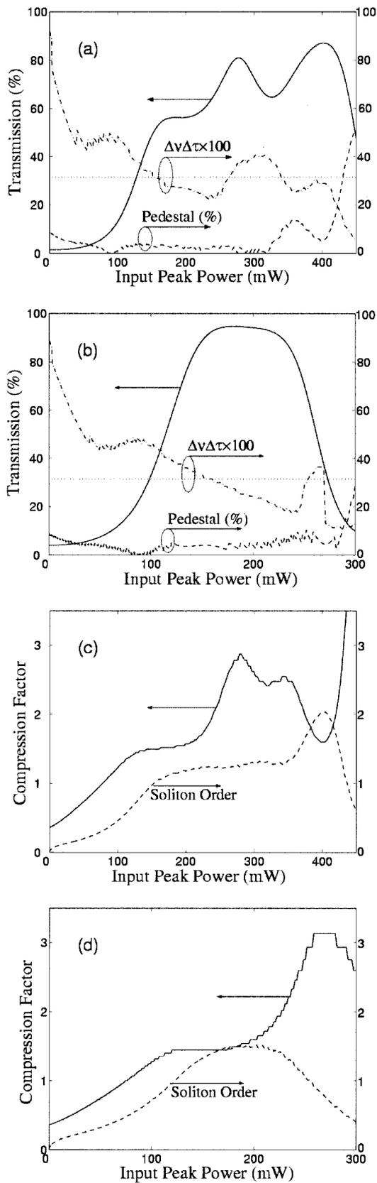
Fig. 2. Switching characteristics of a NOLM and amplifier combination: (a), (c) the coupler has a power-splitting ratio of 56:44; (b), (d) the coupler has a power-splitting ratio of 60:40. In each case, a lumped gain of 10 dB is placed at the input port (outside the NOLM), where  $\Delta\nu\Delta\tau$  is the time-bandwidth product of the transmitted pulse.
