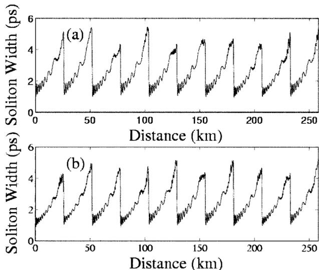
Fig. 10. Pulse width evolution under conditions identical to those of Fig. 9(b) except that the peak power of the input pulse to the first NALM is varied for (a) 487.4 mW and (b) 569.4 mW.
