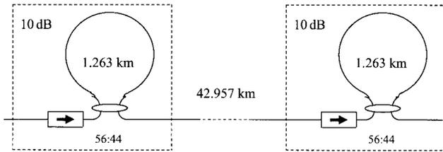
Fig. 4. Schematic diagram of the soliton transmission line.
