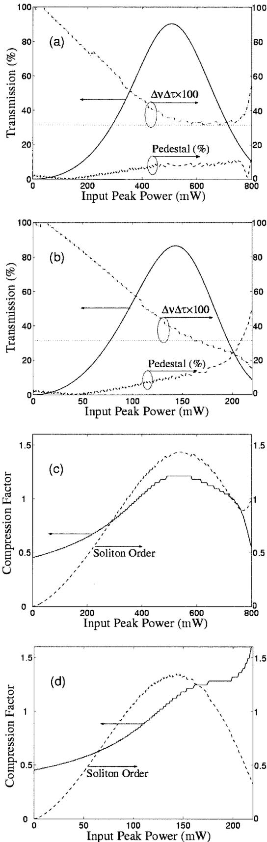
Fig. 1. Switching characteristics of a conventional NALM: (a), (c) with a lumped gain of 5 dB; (b), (d) with a lumped gain of 10 dB, where  $\Delta\nu\Delta\tau$  is the time–bandwidth product of the transmitted pulse.
