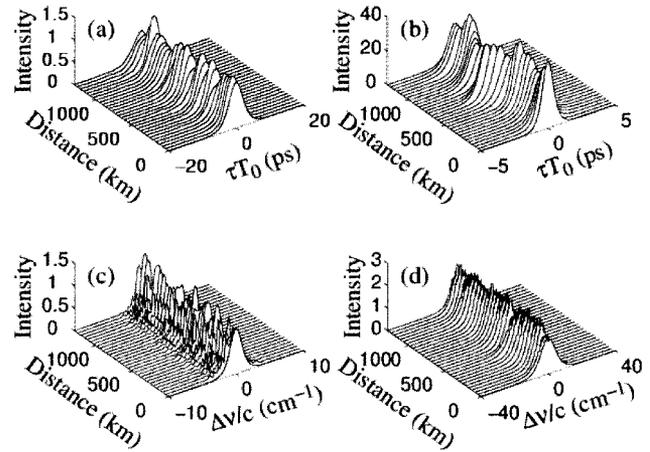
Fig. 5. Pulse shape and spectral evolution through a transmission fiber link with concatenated gain-distributed NALMs, where (a) and (c) are measured at the inputs of the NALMs and (b) and (d) are measured at the outputs of the NALMs.
