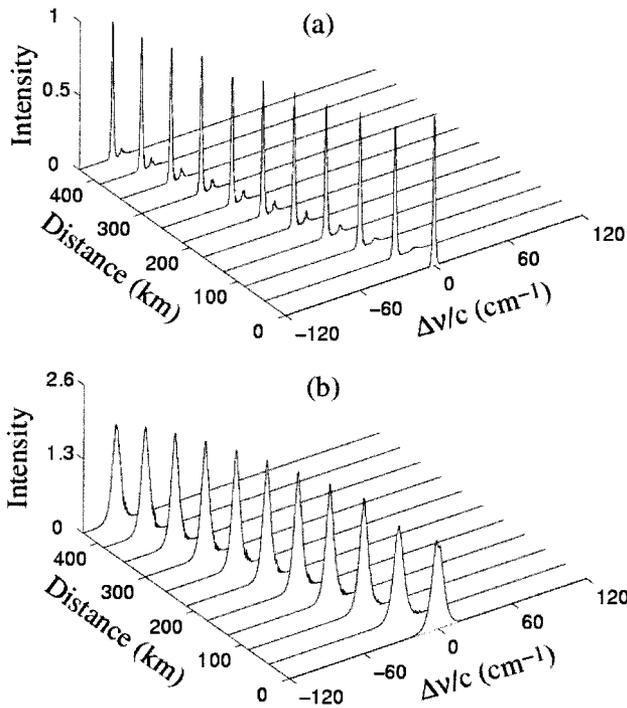
Fig. 8. Spectra evolution under conditions identical to those used for Fig. 5 except that the RSS effect is considered, where (a) and (b) show the pulse spectra measured, respectively, at the input and output of each NALM.
