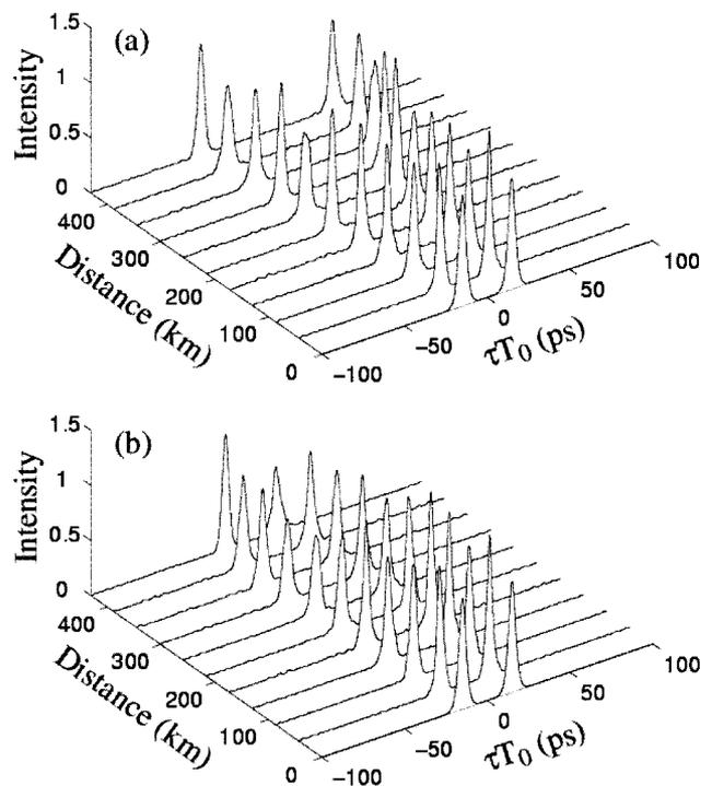
Fig. 7. Interaction of two in-phase solitons initially separated by 30 ps: (a)  $\beta_2 = -20 \text{ ps}^2/\text{km}$ , (b)  $\beta_2 = -10 \text{ ps}^2/\text{km}$ .
