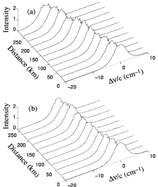
Fig. 9. Soliton spectra measured at the output of each NALM when (a) only the RSS effect is considered and (b) both the RSS effect and the gain-dispersion effect are considered. In both cases, the NALM has a distributed gain of 7.1 dB and the loop length is 2.526 km.
