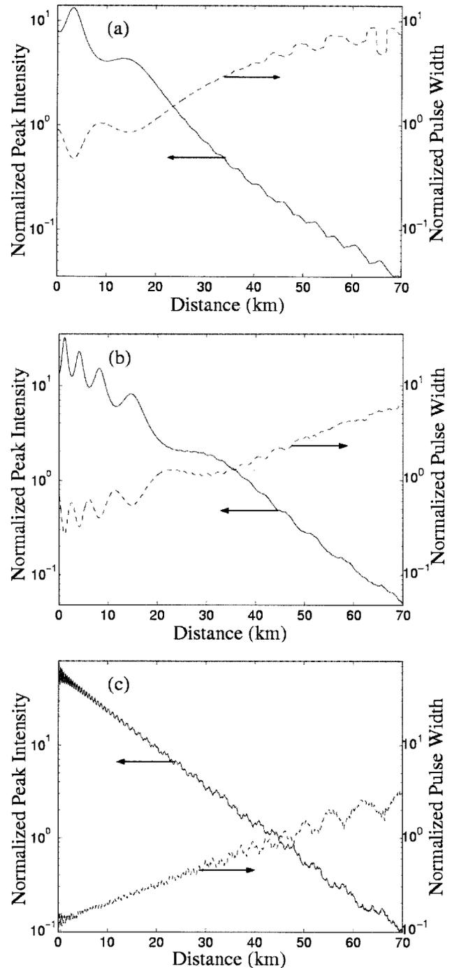
Fig. 6. Evolution of the normalized peak intensity and normalized width of pulses switched from (a) the conventional NALM, (b) the NOLM and amplifier combination, and (c) the gain-distributed NALM.
