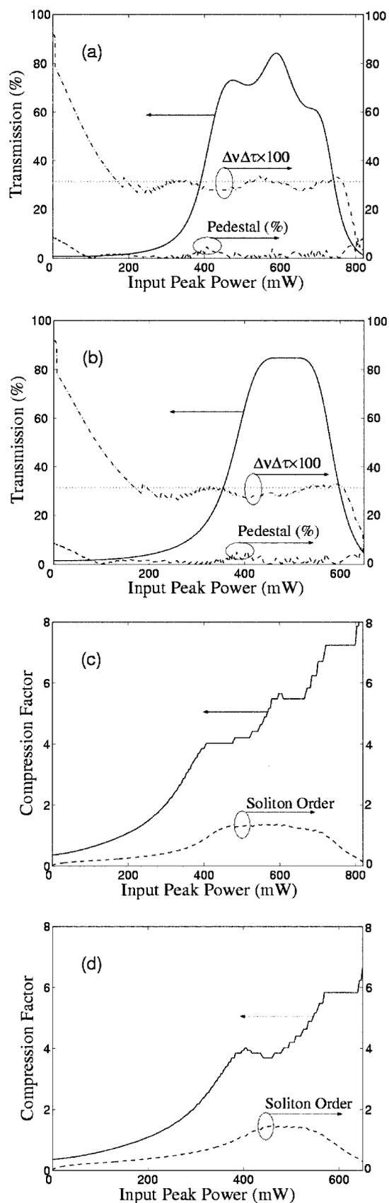
Fig. 3. Switching characteristics of a gain-distributed NALM with a gain of 10 dB: (a), (c) the coupler has a power-splitting ratio of 54:46; (b), (d) the coupler has a power-splitting ratio of 56:44, where  $\Delta\nu\Delta\tau$  is the time-bandwidth product of the transmitted pulse.
