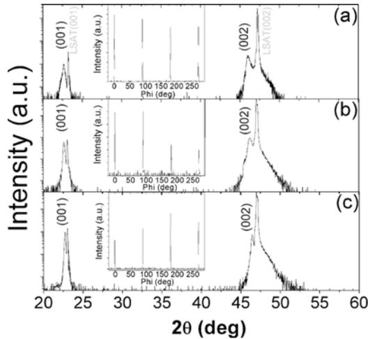
FIG. 1. (Color online) XRD  $\theta$ - $2\theta$  scans of (a) BNBTLaCe, (b) BNBTMn, and (c) BNBT thin film epitaxially grown on CRO(001)<sub>c</sub>/LSAT(001) substrates. Insets are the off-axis  $\phi$  scans of the (202) reflections of corresponding films.
