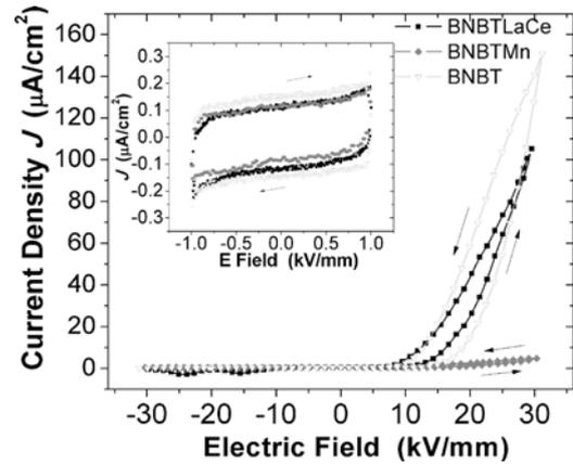
FIG. 3. (Color online) Leakage current density  $J$  as a function of electric field  $E$  for the Au/BNBT-based thin film/CRO capacitors at room temperature. Inset is the  $J$ - $E$  characteristics at low electric field.
