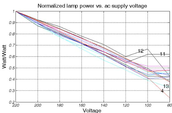
Fig. 4: Normalized lamp power vs. ac supply voltage.
