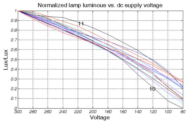
Fig. 6: Normalized lamp luminous vs. dc supply voltage.
