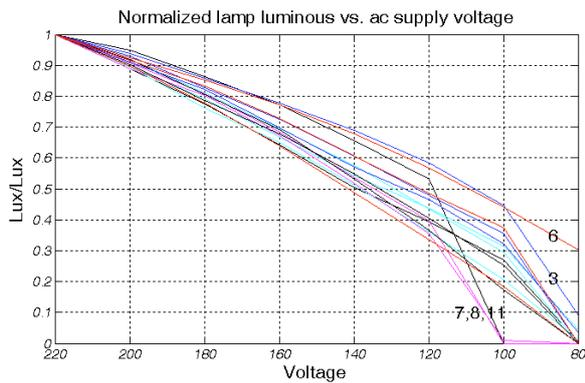
Fig. 3: Normalized lamp luminous vs. ac supply voltage.
