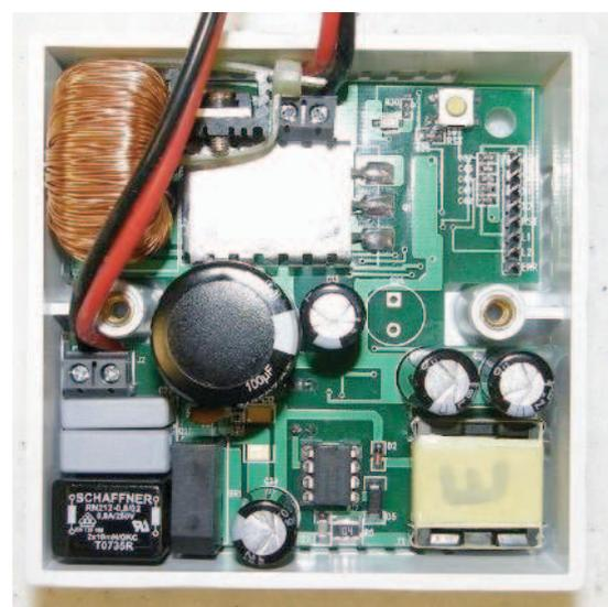
Fig. 14: Evaluation board of 100 W CFL light dimmer
