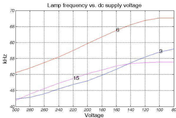
Fig. 11: Lamp frequency vs. dc supply voltage.
