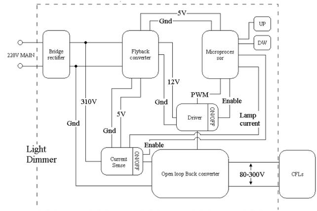
Fig. 13: Block diagram of the light dimmer
