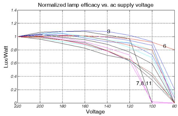
Fig. 5: Normalized lamp efficacy vs. ac supply voltage.
