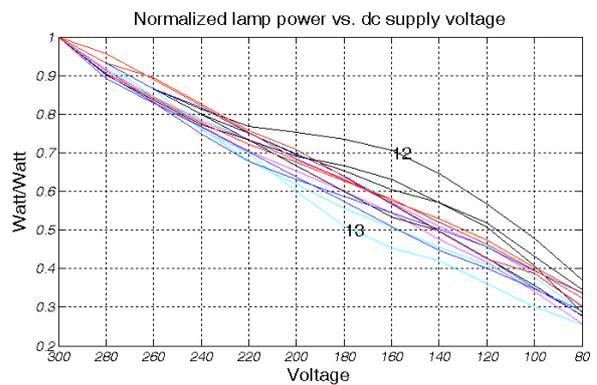
Fig. 7: Normalized lamp power vs. dc supply voltage.
