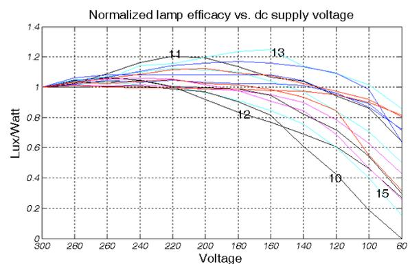
Fig. 8: Normalized lamp efficacy vs. dc supply voltage.
