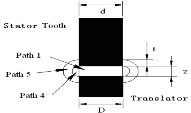
Fig. 4(b) Flux paths from side view
