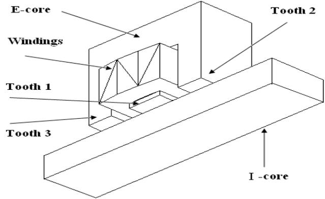
Fig. 2 Schematic of the single levitation coil model
