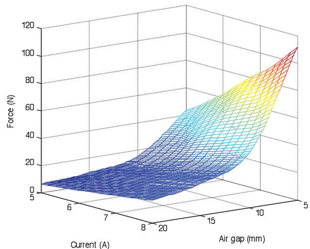
Fig. 5 The diagram of force-current-position by MCA model
