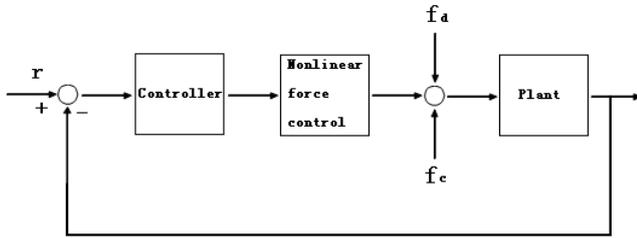
Fig. 6 The control block diagram for single coil
