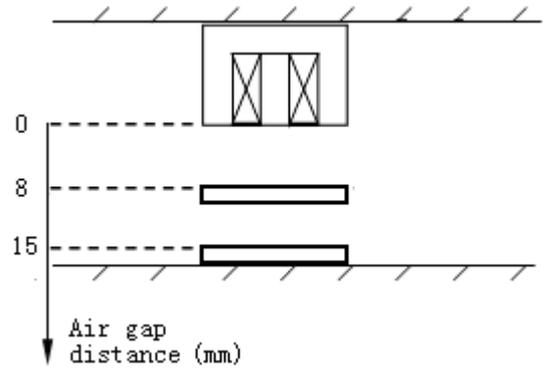
Fig. 7 Schematic of displacement of single levitation coil
