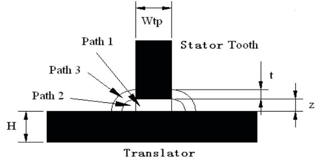
Fig. 4(a) Flux paths from front view
