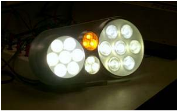
Fig. 9. LED front-light units for vehicle after excitation
