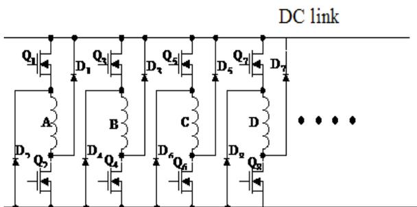
Fig 4: SRG driving circuit and the DC link
