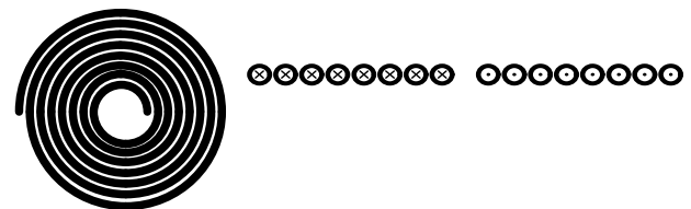
(a) Planform of coil (b) Cutaway view of coil
