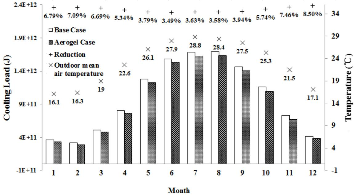
**Figure 7 Thermal performance of silica aerogel window system**
