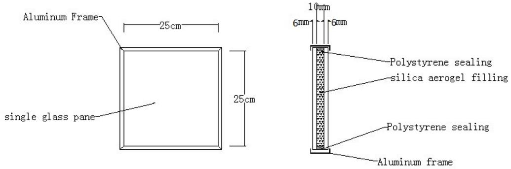
**Figure 2 Diagrammatic sketch of the silica aerogel window sample**
