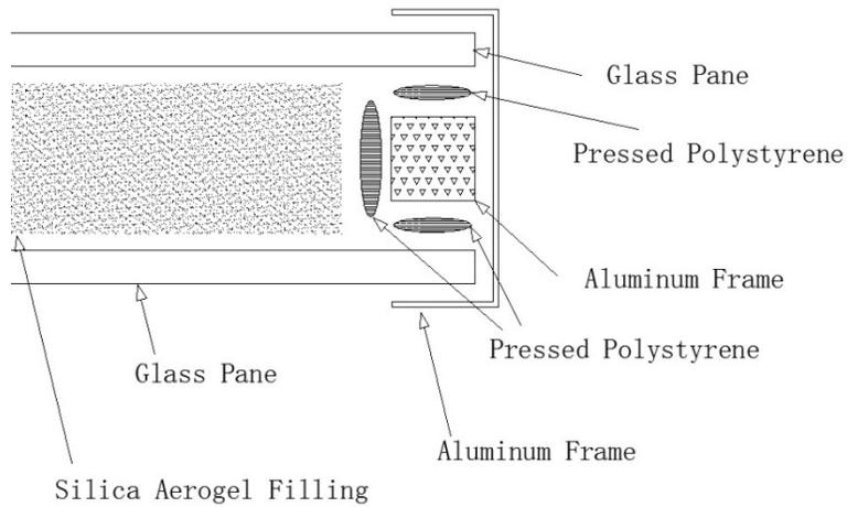
**Figure 3 Schematic diagram of the edge sealing**
