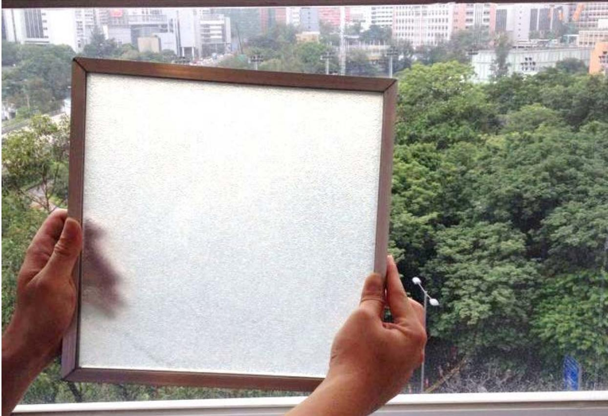
**Figure 5 Appearance of the silica aerogel window sample**
