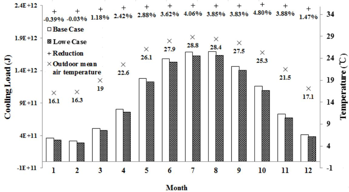
**Figure 10 Thermal performance low-e glazing**
