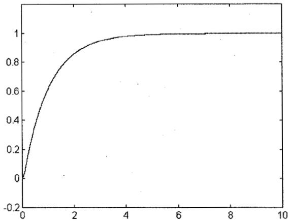
Fig. 1. Step response of the system without applying the proposed algorithm
