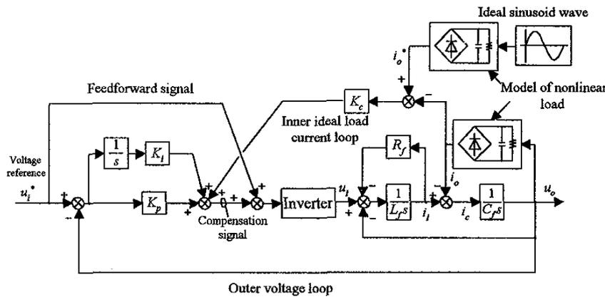
Fig.5. Idealized load-current feedback control scheme to obtain example patterns under nonlinear loading conditions
