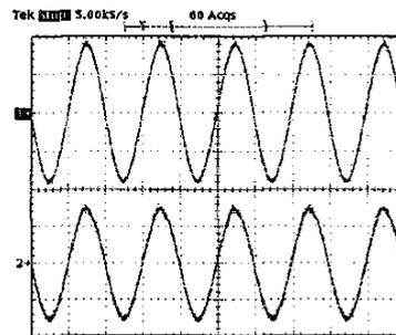
Upper trace: voltage (20V/div, 10ms/div); lower trace: current (4A/div, 10ms/div)
