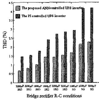
Fig.10. The THD of the output voltage for bridge rectifier loads feeding with different R-C values
