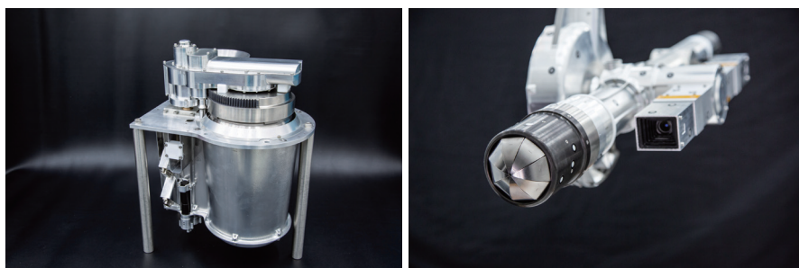
Figure 7. In collaboration with CAST, PolyU developed and manufactured the “Surface Sampling and Packing System” for the Nation’s Chang’e-5 mission, the world’s first fully automated multi-point lunar surface sampling and packaging. The system automatically collected and packed approximately 1.5 kilograms of surface lunar soil samples and returned back to Earth.
