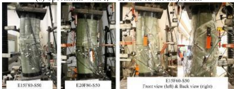
(b) Specimens with e_i = 50 mm on the major axis
