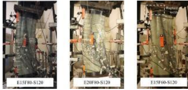
(c) Specimens with e_i = 120 mm on the major axis
