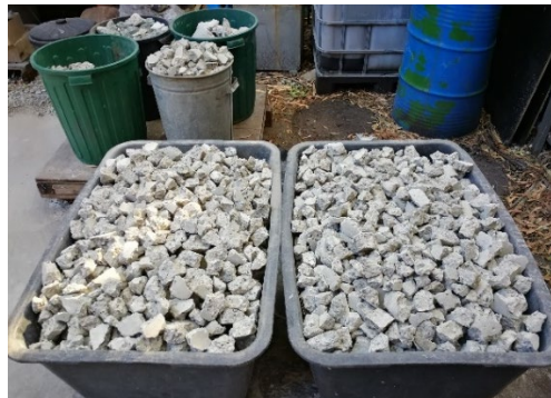
Figure 2. RCLs obtained by crushing concrete columns.
