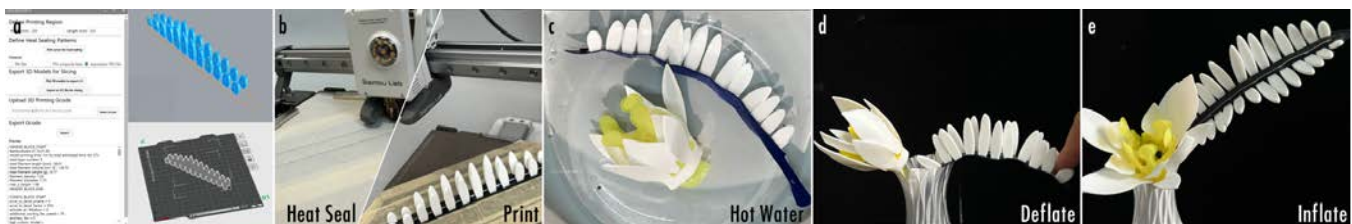
Figure 1: DuoMorph overview. (a) Design tool for modeling and generating integrated G-code; (b) Fabrication of heat-sealed pneumatic actuators (left) and subsequent printing of structures directly on top (right) using an FDM printer; (c) Preshaping the pneumatic actuator with 4D-printed structures in hot water; (d, e) A mimosa-inspired interactive sculpture that folds when touched and blooms when left alone. The flower is also fabricated through a same process.
