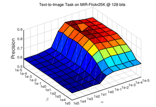
(f) Parameter Sensitivity Analysis of \alpha and \beta on MIR-Flickr25K @ 128 bits Text-to-Image Task
