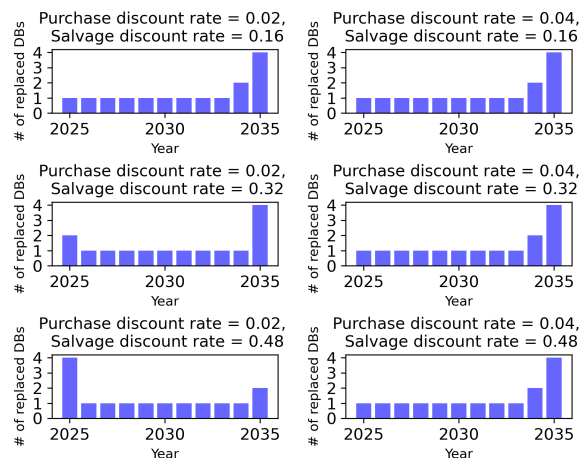
Fig. 8. Fleet replacement schedule with different purchase discount rates and salvage discount rates (the original DB fleet before ZEB transition is 15).
