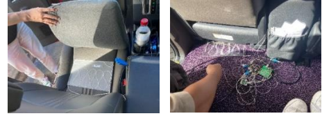
Fig. 16. Application of the proposed optical fiber sensor for HRV monitoring and fatigue condition detection in vehicle driving.
