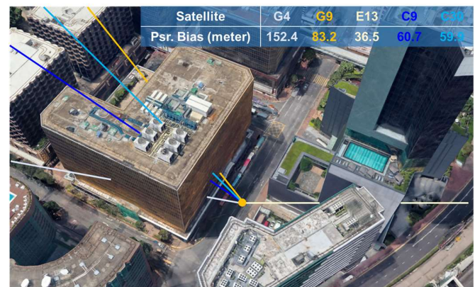
Fig. 1. Demonstration of satellite signal receptions in an urban canyon of Hong Kong. The receiver position is marked as a yellow dot. The colored lines are Line-of-Sight (LOS) transmission paths of satellite signals. A list of the pseudorange observation error (denoted as Ps. Bias in the figure) is given in the table in the upper right corner.
