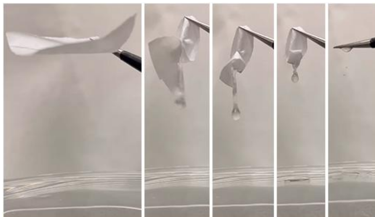
Supplementary Fig. 1 The procedure of TSN web waste dissolving in N,N -Dimethylformamide (DMF) at ambient atmosphere.
