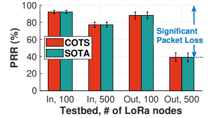
Fig. 7. Packets under logical channel interference suffer from significant packet loss.
