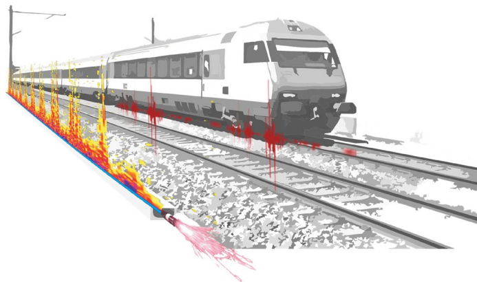
Fig. 16 Schematic diagram of changes in sensing fiber optic cable signals when a train passes [144]
