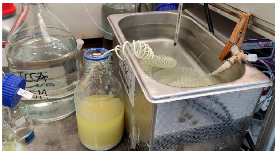
Figure 2. A photo of the setup employed for the perchlorination of p -cresol to 2 .
