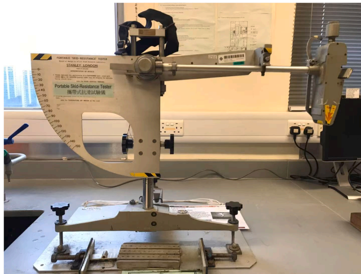
Fig. 8. The British pendulum friction test.
