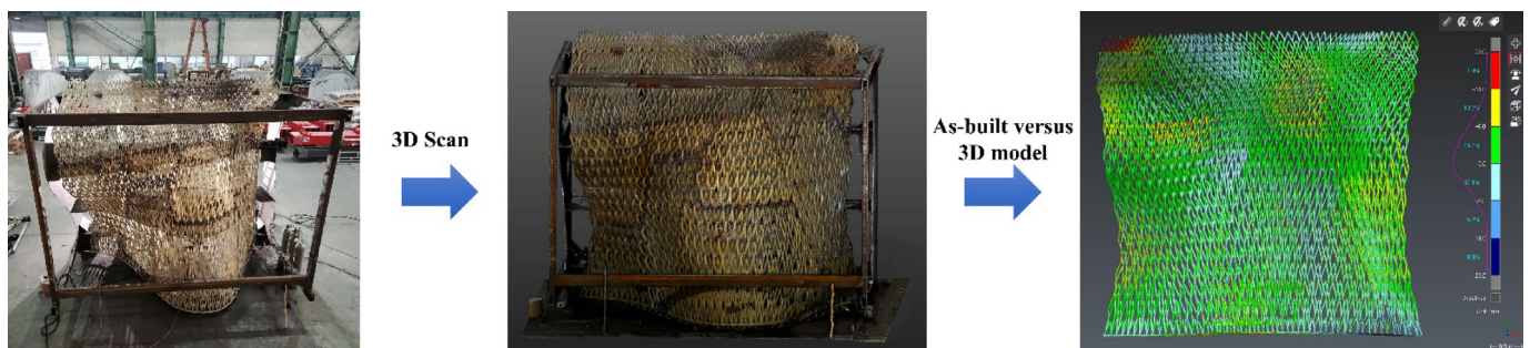
Fig. 24. Post-assembly 3D scan to ensure overall dimensional integrity.
