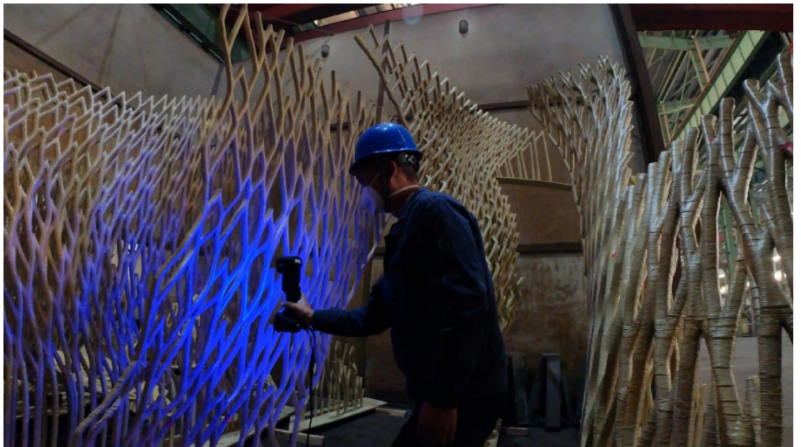
Fig. 22. 3D scans and visual inspections.
