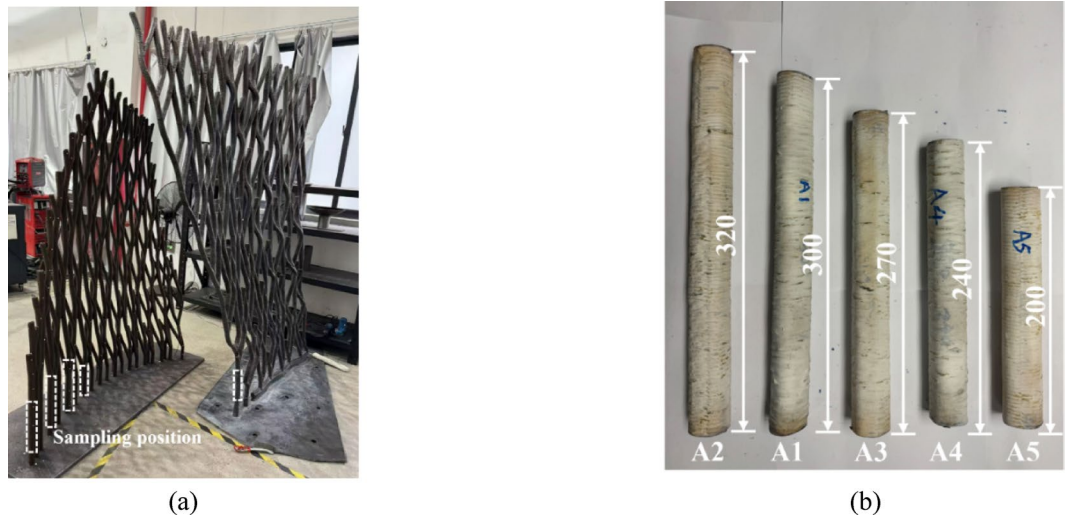
Fig. 16. Compression test: (a) sampling position; (b) test specimens.
