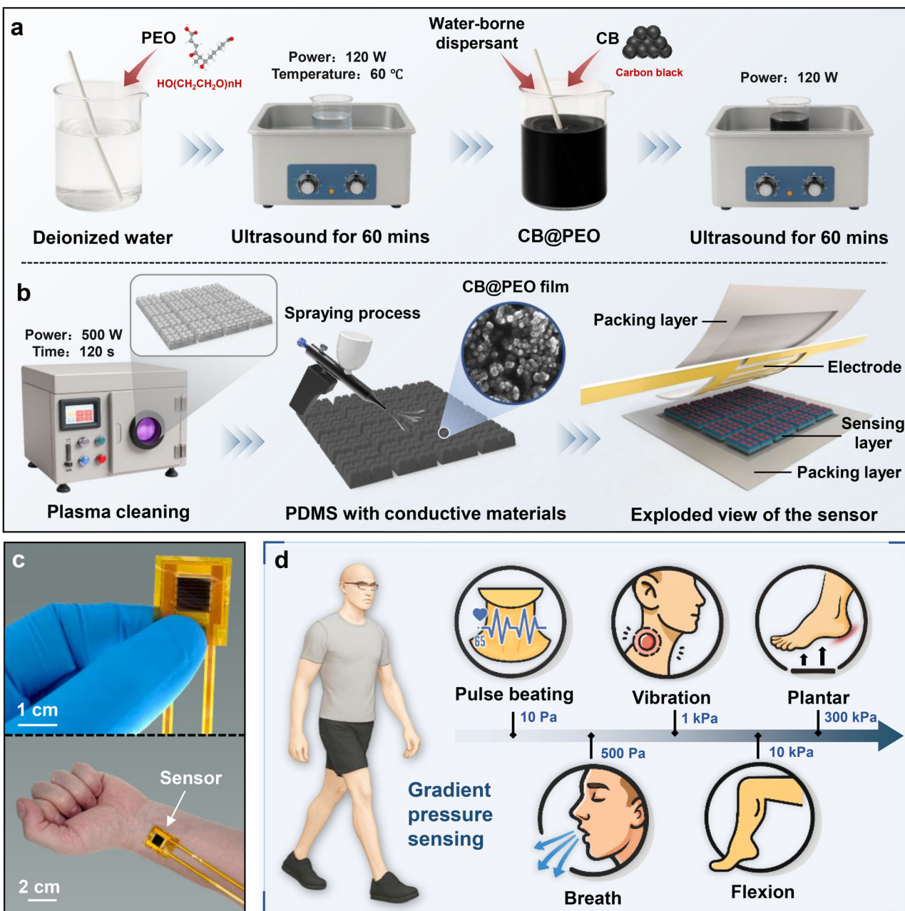
Figure 3. Fabrication of the pressure sensing layer and sensor packaging. a) Process flow for the preparation of the conductive material. b) Spraying of the pressure sensing layer and sensor assembly. c) Image of the pressure sensor and its installation on the wrist for monitoring. d) Physiological health monitoring using the pressure sensor across a wide pressure range from 10 Pa to 300 kPa.
