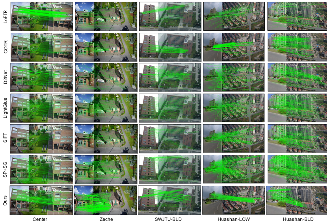
Fig. 7. Aerial-ground image matching results. Our method produces more accurate matches across various scenarios, outperforming both direct matching and mesh-based methods. These results highlight the effectiveness of our approach in bridging the modality gap between aerial and ground images.
