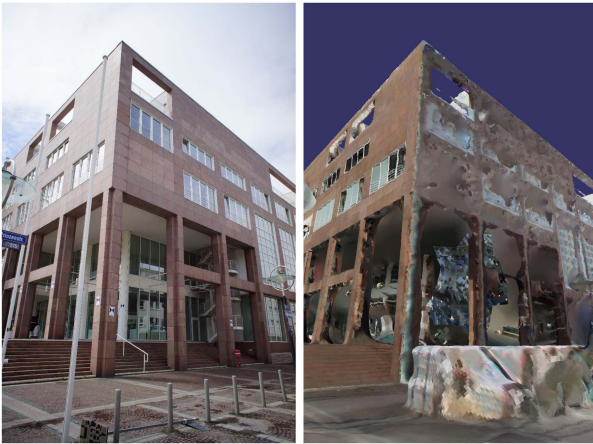
Fig. 5. Difference between synthetic and ground images. These errors arise from deformations, texture loss, and noise in the mesh model, leading to discrepancies between the synthetic and actual images.
