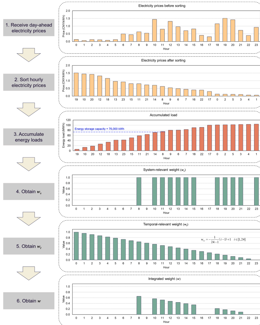
Fig. A4. An intuitive example of calculating the weights of the proposed dynamically weighted error (DWE). Step 1: Receive the hourly electricity prices ahead of a day. Step 2: Sort the electricity prices in a descending order to get a sorted series of hour indices. Step 3: Accumulate the hourly energy loads in the order of the sorted hour indices until the accumulated load is just higher than the energy storage capacity. Step 4: Set value 1 at the hours of accumulated energy loads, and set value 0 at other hours of a day, to obtain the system-relevant weight ( w_s ). Step 5: Set values at hours based on Eq. (3) to obtain the temporal-relevant weight ( w_t ). Step 6: Calculate the Hadamard product between w_s and w_t to obtain the integrated weight ( w ) of the proposed DWE.
