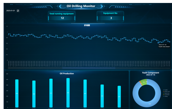
Fig. 17. Oil drilling monitor interface, where the pie chart indicates the fault probability of different components
