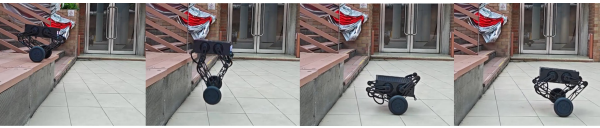
Fig. 25: Robot jumps down from a 40 cm platform.
