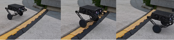
Fig. 24: Robot traverses a 3 cm speed bump.
