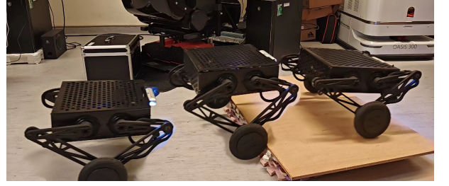
Fig. 26: Robot automatically jumps onto a 10 cm step.
