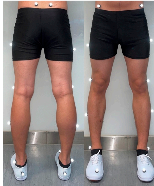
Figure 2. Marker set with sixteen retro-reflective markers.
