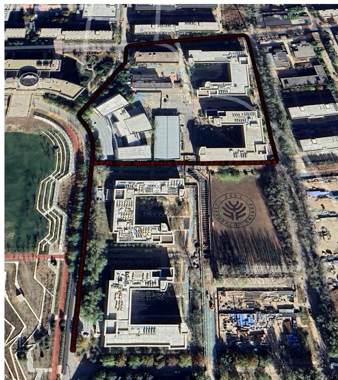
Figure 10. Scene map and trajectory layout for Experiment 2, visualized in Google Earth. The trajectory shown represents the ground truth, collected using the Vision-RTK 2, with red circles denoting pedestrian positions sampled at one-second intervals.
