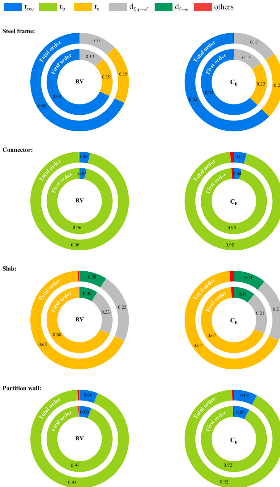
Fig. 6. Global sensitivity analysis of [15-yr, 25-yr] scenario. RV represents residual value, C_E represents environmental cost. r_{rec} represents recycling rate, r_a represents repair rate, r_b represents replacement rate, d_{f,m \rightarrow f} represents distance from the material manufacturing factory to the prefabrication factory, and d_{f \rightarrow s} represents distance between the prefabrication factory to the project site.
