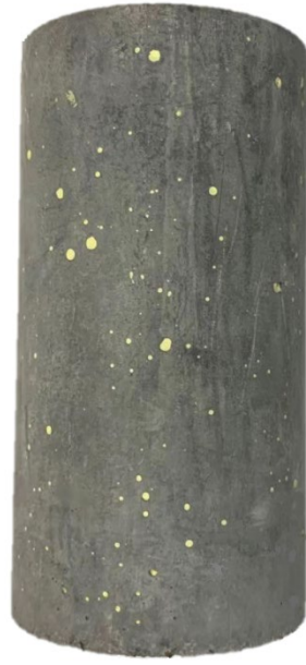
Fig. 1. Surface patching using gypsum for specimens of triaxial compression tests
