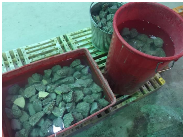
(a) RCLs submerged in water
