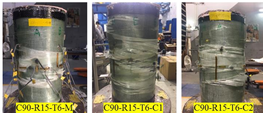
(c) CCFFT specimens (RCL mix ratio = 15%, 6-ply FRP tube)
