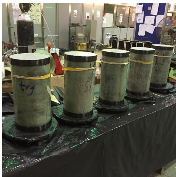
(c) End strengthening with CFRP strips
