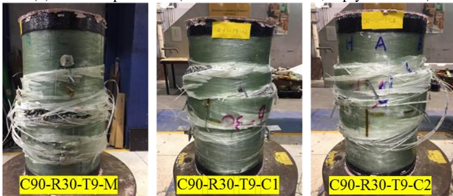
(e) CCFFT specimens (RCL mix ratio = 30%, 9-ply FRP tube)
