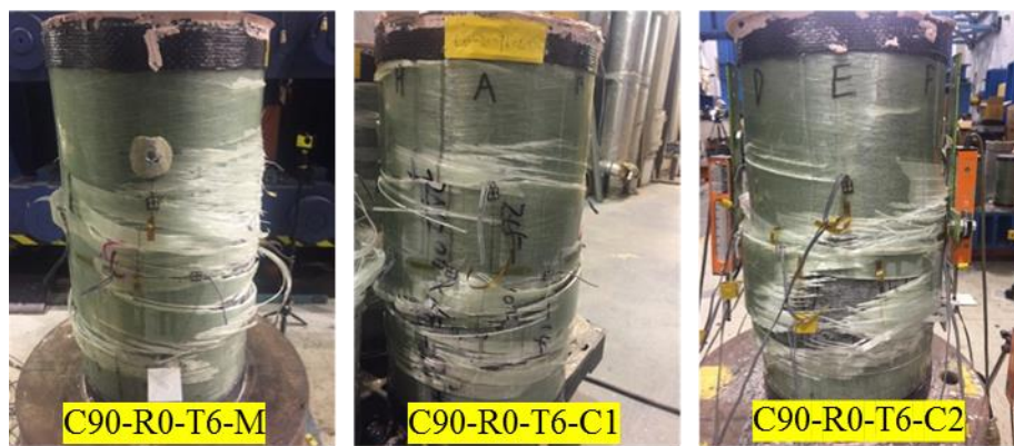
(b) CCFFT specimens (RCL mix ratio = 0%, 6-ply FRP tube)
