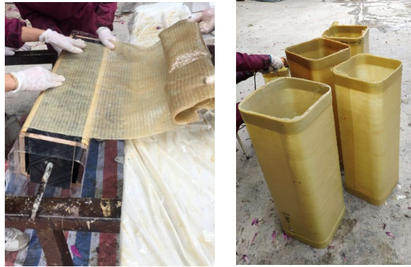
Fig. 3. Fabrication of GFRP tubes
